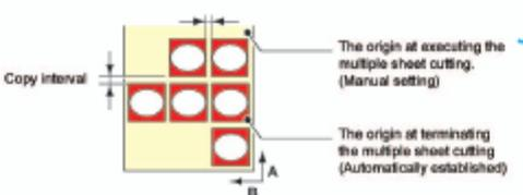
The origin at executing the multiple sheet cutting. (Manual setting)
